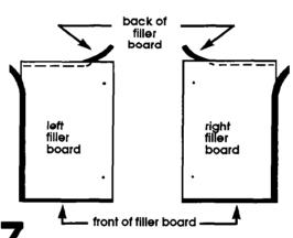
■ Apply 9.5 mm (3/8") seal strips to bottom and outside of filler boards. The top seal goes on back side of filler boards.
